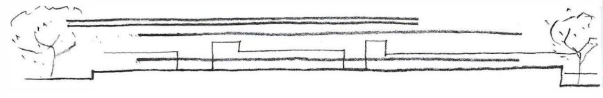
Translation of the design concept The side walls are detached from the floor and roof, allowing each horizontal and vertical element to be read as an individual entity enclosing the space
